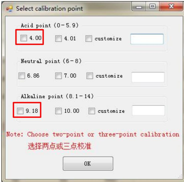
4.First calibrate in a solution with a pH of 4.0. After the data is stable, click 'auto matching', Then clean the sensor probe with water and calibrate in a solution with a pH of 9.18, After the data is stable, click 'auto matching', After the data is stable, click 'auto matching'. Then click 'Confirm calibration'. Click to '确定'in the pop-up window
